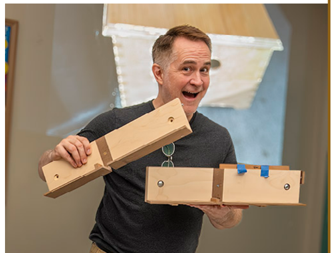
Jonathan showed off his box finger-joint jig (plans can be purchased from https://tinyurl.com/3wubp4jd ) with interchangeable finger widths (e.g., 1/8", 1/4") and the ability to fine tune with the turn of a screw.
