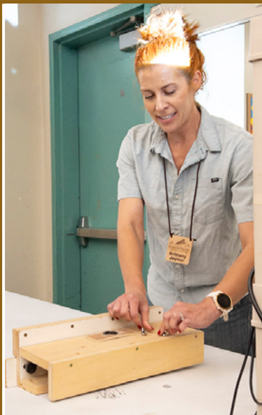
Brittany Joyner attaches this router table fence onto her tablesaw fence to provides the proper fence when using her router on the table Saw extension. This also has a hole to attach her Shop-vac to remove the created sawdust.
