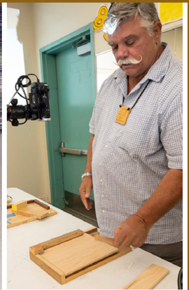
Jim Baldrige shared the jigs used to make the teen boxes for the toy build. The assembly requires very tight tolerances and alignment, and the jigs he uses accomplishes that.
