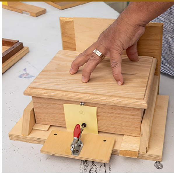
Jim Baldrige shared the jigs used to make the teen boxes for the toy build. The assembly requires very tight tolerances and alignment, and the jigs he uses accomplishes that.
