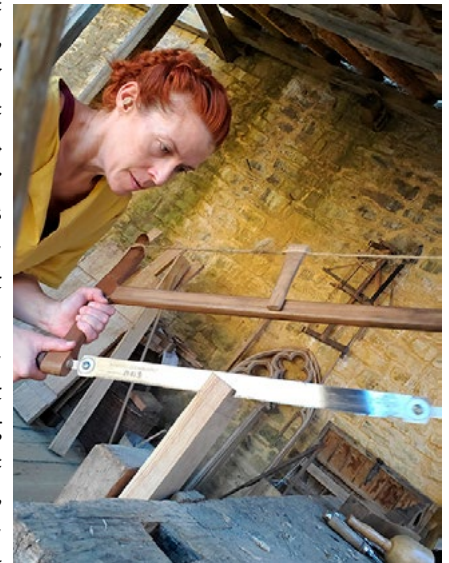
Sawing finger joints for the chest’s lid
