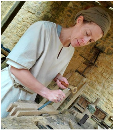
Chiseling on the lid's frame to receive the slats
