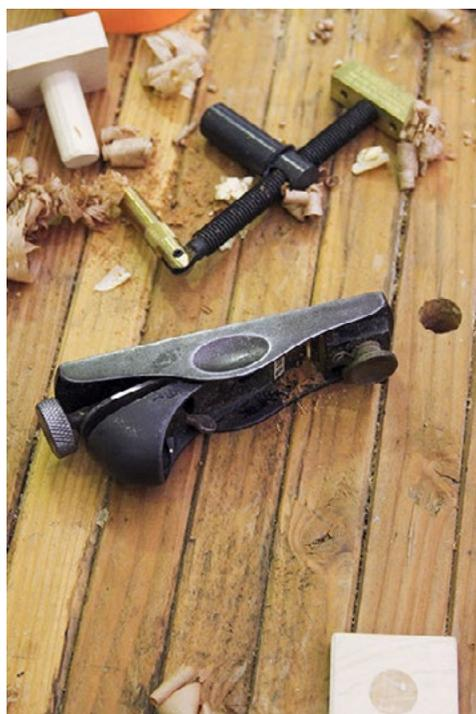
Steve said that you want to read the grain before starting to plane so that you do not lift the grain and get tear-out. You also want to transfer your hand pressure as you pass your plane across a cut, starting with downward pressure at the front of the plane and shifting that pressure toward the back of the plane as you finish the cut.
