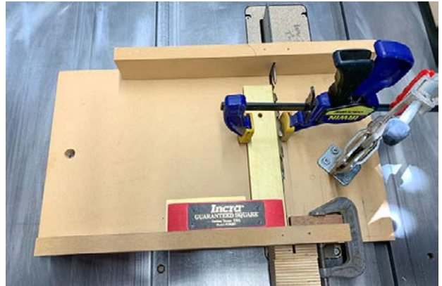
A small parts crosscut sled that includes a toggle clamp to keep parts from flying off the sled.
