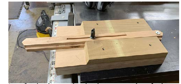
A jig for the disc sander that lets you sand perfectly round parts.
