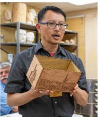
Keenan showed a tool chest. The case is dovetailed and made from figured cherry. The lid was made using frame and panel construction. He uses the chest for planes, saws, and scrapers. There is a drawer for chisels and measuring tools. It was finished with Rubio Monocoat.
