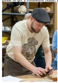
ways to sharpen your tools, but whatever method you use should be fast and easy so that it does not deter you from doing the sharpening. He uses the Veritas Mark I honing guide. It is simple, and he likes that it can handle skew blades and other weird stuff. There are sideclamp guides that will work well for straight blades.
