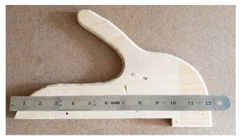
Lastly, this design came from Bob Rennie and is being shared by Gary Coyne. This design makes it easier to grip as it follows the angle of the hand. Like the Sabatino design, these are cheap and easy to make, so if the bottom is cut on the table saw blade, no problem. Plus, like the Sabatino design, it's safe to use this to push small pieces away from the spinning saw blade. The general concept of this design
