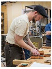
slight angle (or not at all). He uses a triangular burnisher with a narrow edge.
