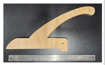
This is the kind designed and used by Ron Sabatino. it has the same dynamic of pushing, but it extends the front section significantly so that the user can control the far side of what you're pushing and prevent it from lifting off the table. Made from scrap cheap plywood, they are easy to make a bunch of them.
