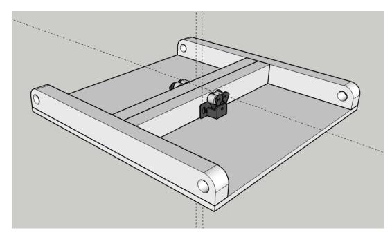
7. Attach the hinge pieces to the underside of each top piece. Make sure that the pattern of the squares of the two sides line up properly. [It's best if the lighter of the two woods is in the bottom right corner – see drawing]. The "outside" edge of the hinge piece should be 5 3/4" from the center of the top.
