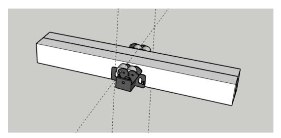
5. Route the length of each of the hinges along one side with a  $\frac{1}{2}$ " round over bit
