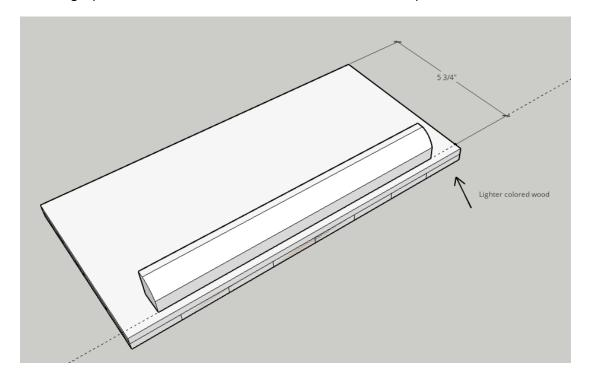
8. Lay the top pieces face down, and lay the bottom in place, lining the edge of the hinge piece, with the bottom edge. With the  $\frac{1}{4}$ " drill bit, drill through the holes in the side pieces into the hinge pieces.
