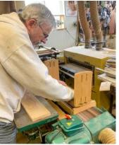
George Leach took club members on a virtual tour of his guitar shop (phoenixguitarco.com). He showed several of the jigs he uses to make guitar parts, including forms for shaping the sides, a jig he made for a long belt sander to shape the radius on the underside of fingerboards, and a jig that is used to cut soundboard pieces to length, width, and thickness,
