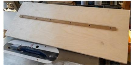
Because of the screws in the mitre bar, the mitre bar had minor bulges at those locations and didn't glide easily in the mitre slot. To fix this, I ran a standard square Nicholson file along both sides of the length of the mitre bar until it fit just right.
