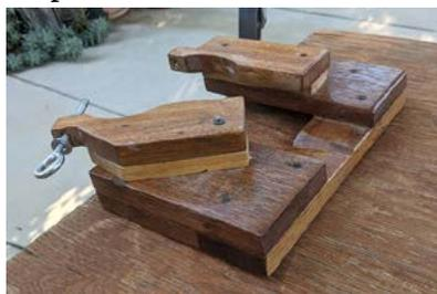
low clearance for the cord and has a locking screw going through a T-nut. He uses a foot switch to power it on and off as the normal switch is covered when the tool is mounted
