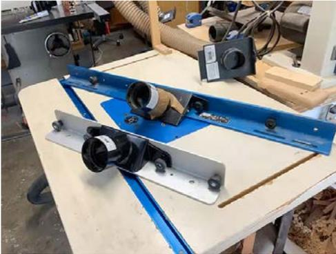
Jeff Bremer described a problem he was having with the dust collection off his router table fences, due to the vacuum hose pulling on the fence's dust shroud and opening gaps.
