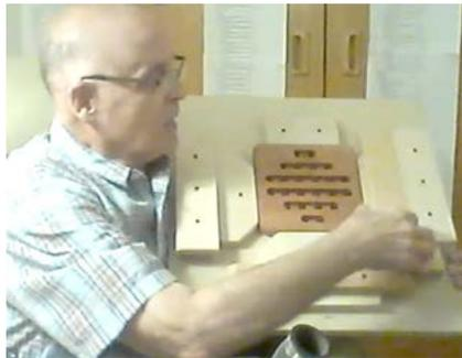
Greg Golden showed a crosscut sled he made that has toggle clamps mounted on the fence on either side of the blade to hold down work pieces. He also showed
