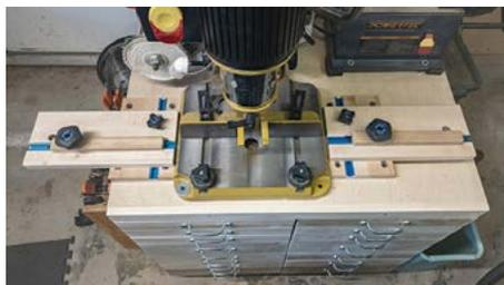
and end-stops on his benchtop mortiser. Gary is a big fan of stops on his tools and this does the trick for his mortiser. This uses T-track on table extensions to hold stop blocks on either side of the mortiser
