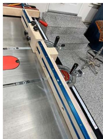
made for his tablesaw, using paired Inca miter gauges. He used T-track to hold the stop blocks on the fence. His stop block uses two T-bolts and knobs on the top and two on the face to lock it into place, as he has found that flip-down stops
