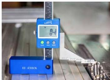
But there are times when it's important to be exact. For example, if you want to set the exact height of a dado blade to provide a dado that is JUST deep enough to receive the edge of a board.
