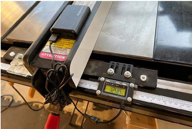
There is a quicker way to calibrate: simply place a 2" block between the blade and the fence and press the Calibrate button for 3 seconds. While not as accurate, it's faster than above.
