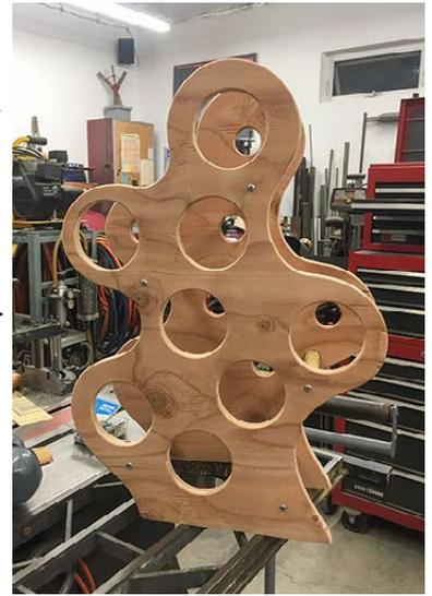
Searching through my collection of plywood scraps, I came across a piece that was flat, 3/4" thick, and not too crappy (as the wood was construction grade), and not the kind of wood my woodworking chums usually use. It was a 2' x 4' piece and cutting it in half left me with my 2' x 2' starting size. Scaling the design to the wood, I was able to fine-tune the number of holes and placements, creating what I thought was a nice design.
