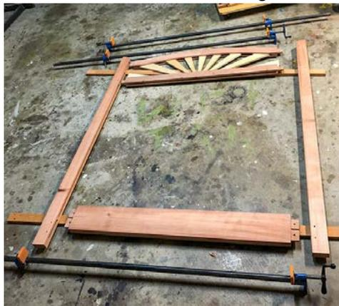
get them aligned right when gluing them in place (I used Titebond III, both for its outdoor application and longer open time). I set the bottoms of all the pieces in first, then put the arch stile in place. Once the glue had set, I went back and drilled holes to pound in 3/16" dowel to lock each in place – I wanted a mechanical fastener in case the glue fails in the years ahead. Another piece of 1/2" thick cedar was cut to insert into the frame on the diagonal to resist future sagging.
