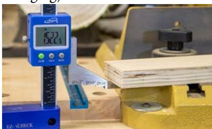
The crenulated bottom of the measuring foot lets you locate the center of a router bit (1/4", 3/8", and 1/2" shafts) against a router table's fence. The EZ-Check can lie flat on its back
