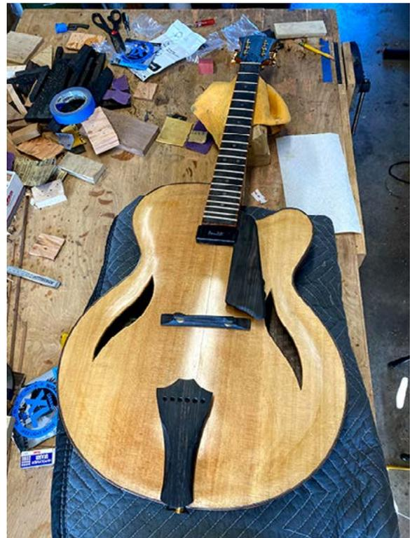
slots for the strings, each file matching the diameter of the respective string. The tuners are now attached.
