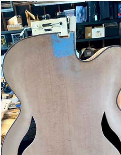
rubbed off, gently carve that away with a chisel, wash, rinse repeat until the fit is good. This procedure can take hours to get right, but once complete, the neck is glued on and now we REALLY have a guitar!
