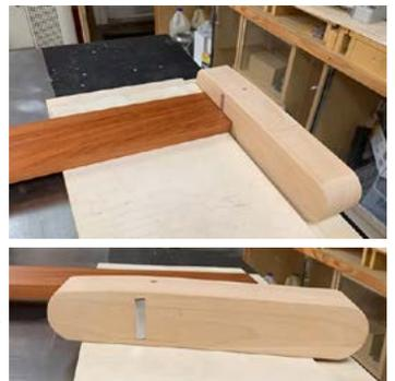
Marc Collins showed a zero-clearance "mega fence" he made for his tablesaw, using paired Incra miter gauges. He used T-track to hold the stop blocks on the fence. His stop block uses two T-bolts and knobs on the top and two on the face to lock it into place, as he has found that flip-down stops
