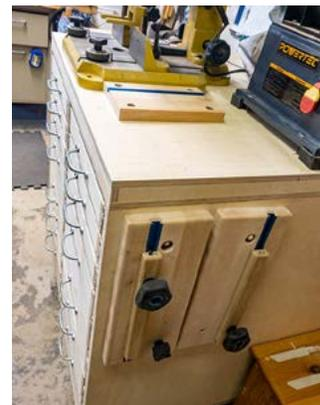
and extend over the base of the mortiser or can rotate 180° so that the stop can be far away from the mortise bit. Plus they also support longer boards. He uses a round head screw in the end of either stop block for fine adjustments. Once he's done, the "wings" of this system can be placed on the end of his mortise bench.
