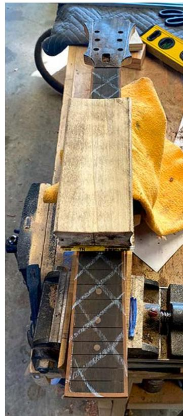
I have a piece of 80 grit paper adhered to the concavity so that I can sand the fingerboard from a flat piece of wood to a surface that has a slightly rounded profile (this adds to the playability of the guitar). Frets are now cut to size and pounded in using a dead blow hammer. I used gold colored fret wire which will match the gold tuners and contribute to the warm look of the guitar.
