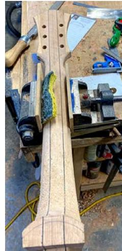
so thin that strength and durability are compromised. Raspers, files and a spokeshave are used, and hopefully at the end I have a smooth surface that fits nicely into the hand of the player.
