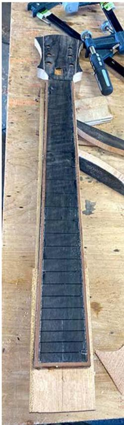
With the fretboard attached I can start the process of bringing the neck to the desired shape. This takes patience and should be done carefully as this is one of the player's primary points of contact with the guitar. It should be thin and round enough to be comfortable, but not
