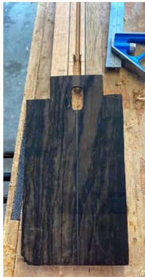
and then a template is used to draw the shape, which is rough cut on the band saw and finished on the spindle sander. The whole thing is then thickened to 16mm (or whatever is called for by the tuners to be used) and then the tuner holes drilled. Last, the truss rod is installed and covered over with a mahogany shim.
