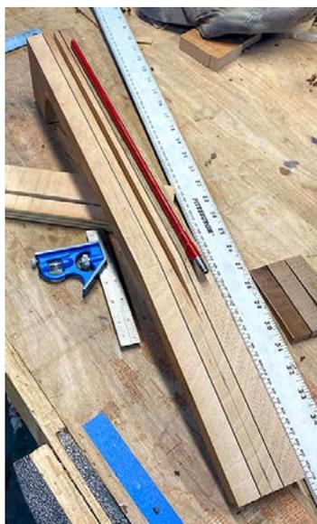
thing together, alternating the two pieces of fiberboard between the three pieces of mahogany, creating a triple decker sandwich. It should be noted that by flipping the flat sawn pieces 90°, they are now quarter sawn resulting in a super strong assembly.
