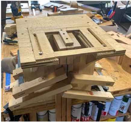
Then it's on to the tenon. Using a jig equipped with a 4.5° ramp to match the neck, and a template, I use a router to cut the tenon into the heel of the neck. This is only done after I've cut a couple of test pieces (both mortise and tenon) to assure the two will go together. Thanks to Chuck for helping me build this jig!
