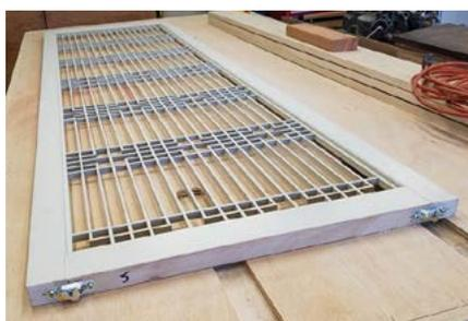
These are a closer look at the detail of the latticework. All the sticks are made of 1/2" x 3/16" Douglas Fir. I believe the outer frames are also DF, measuring 1.2" x 2".
