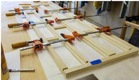
I made Fascias to cover the headers, lights, rollers, and tracks. We decided they needed to extend about 10" above the Header, and about 3" below. The wood is 3/4" solid poplar. Each piece is rabbeted on the back to allow space for the plastic. The middle area joints are just glued and the vertical end pieces are joined to the horizontal pieces with wood screws and
