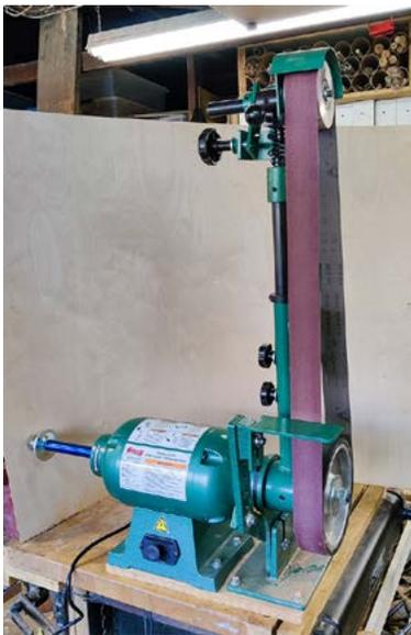
Assembly was quite straight-forward; it took me 30 minutes (and machine assembly is not my long suit). Older reviews mention tracking issues but it appears Grizzly has addressed them. Its only drawback is the tool rest: the usual 2-piece articulated monstrosity has trouble holding a setting under pressure. As I design and build a supplemental rest which will allow precise, repeatable work. I'll feature its build in a future issue.
