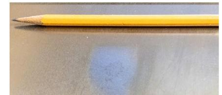
The slight discoloration you may see in the last picture is a both a bit of film left on the sanded area as well as the surface is a bit more polished than the surrounding areas. But any texture or change caused by the rust is gone.
