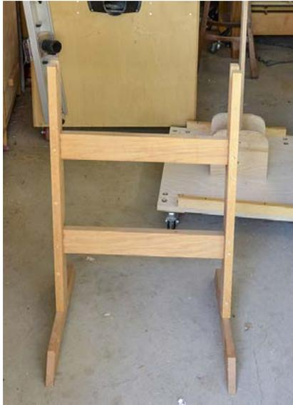
As you can see from the photo, the uprights are notched and can accept various cross members for various tasks. At one time, before I built a cart to hold my thickness planer, I had it mounted on a piece of  $\frac{3}{4}$  inch plywood that had two cleats under it. The cleats were notched, and two sawhorses were used to hold the planer while in use. When not in use, it was housed in a drawer in the cabinet on the left of the photo.
