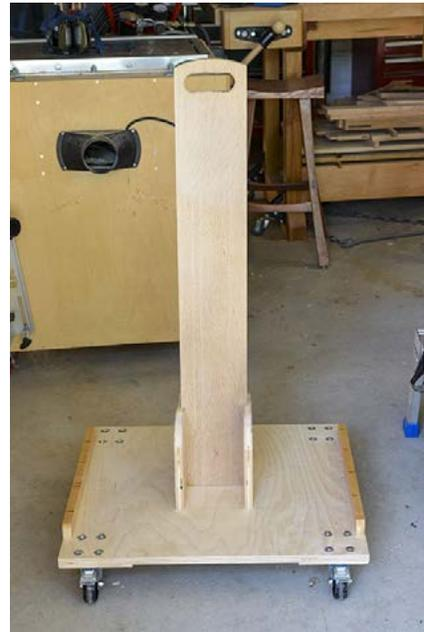
two plywood panels. The panels are screwed to the base and the handle to the panels.
