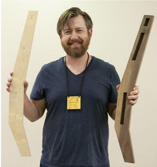
shapes of the outer leg surfaces. This changed the stub mortises cut the previous day to through mortises. The rough bandsaw cuts were smoothed by pattern routing and finished with spokeshaves, scrapers and
